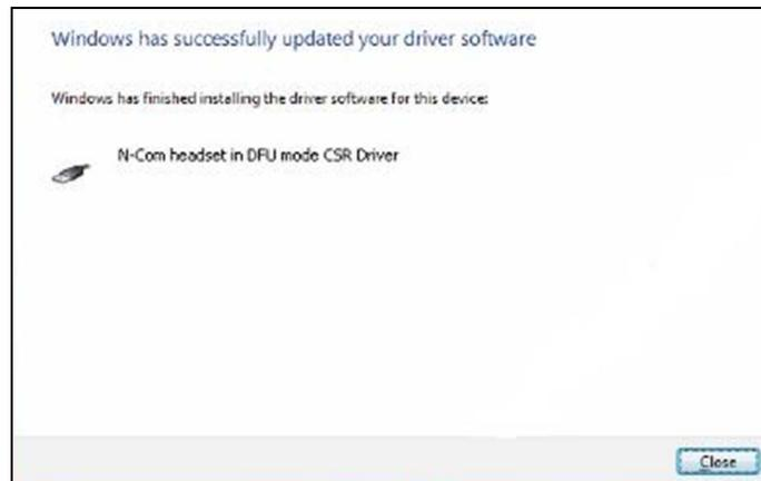
17. The N-Com Wizard will re-start automatically at the end of the installation of the USB drivers. You will then be able to proceed with updating the firmware as described in steps 3 and 4 of the procedure.
